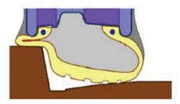
Casing plies inside the tyre are broken by a severe impact due to hitting a pothole or a kerb.
